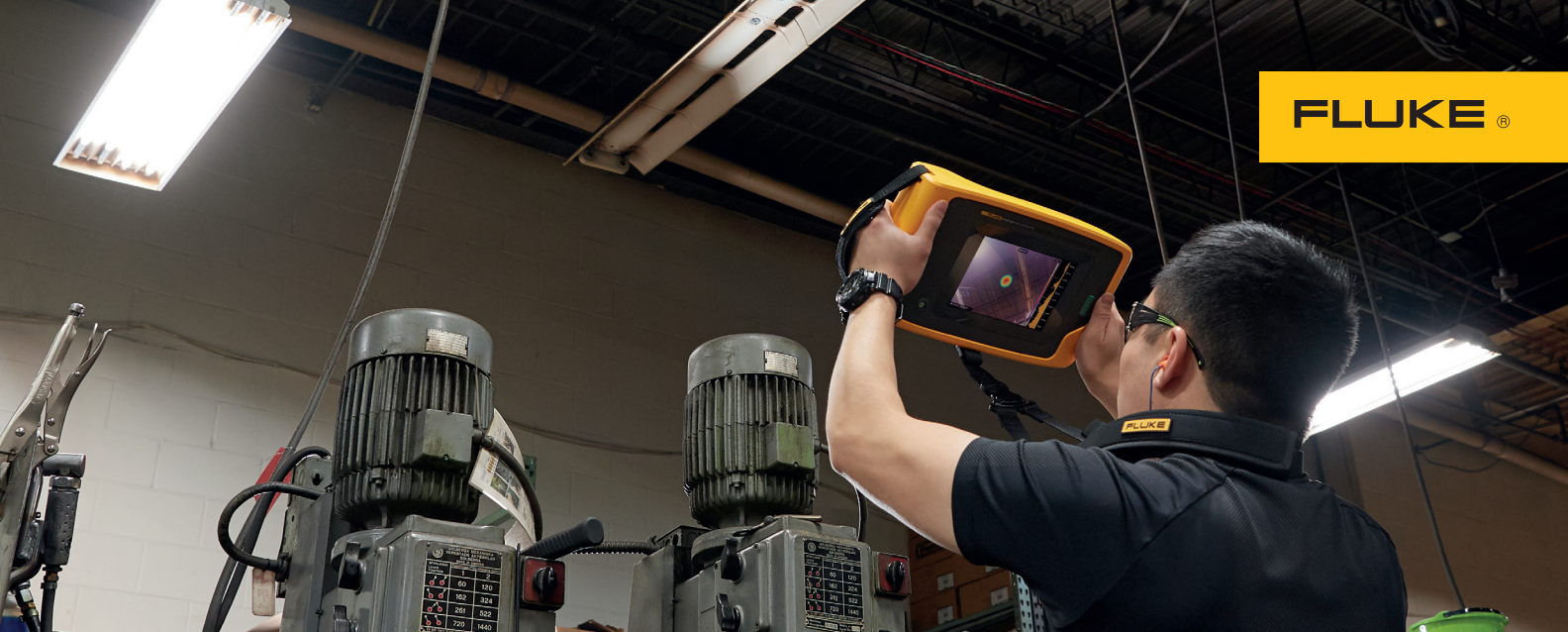
Inspecting compressed air lines with the Fluke ii900 Sonic Industrial Imager
